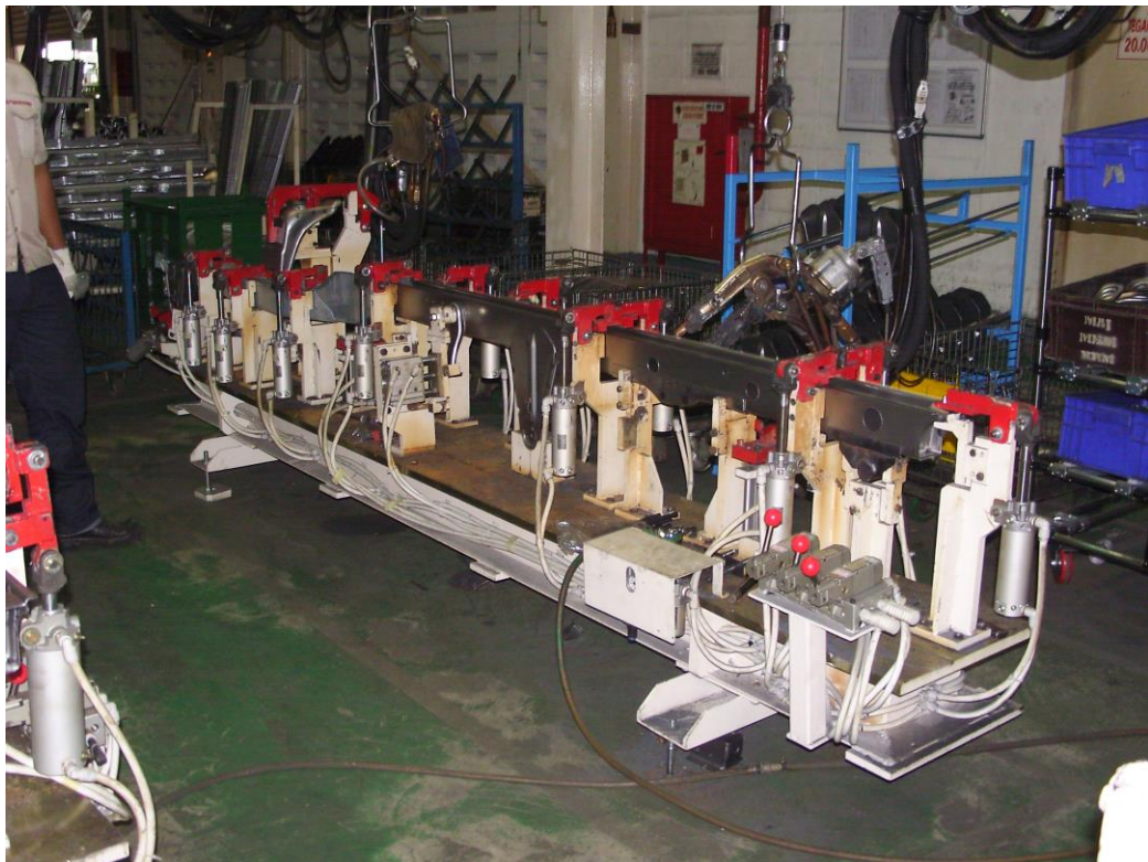
FRAME COMP WELDING JIG
